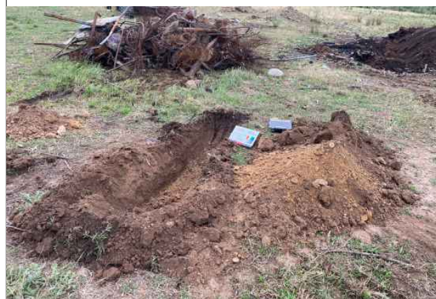
Photograph 12 – TP02 ground conditions, noting natural ground encountered approximately 0.2 m BGL.
