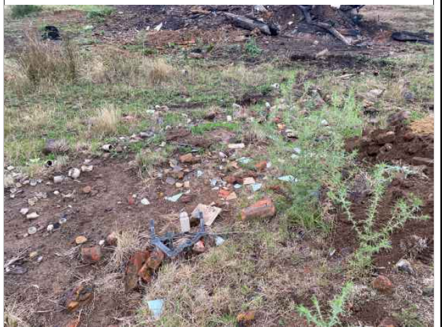
Photograph 8 – C&D waste (tile and brick fragments, electrical insulators) at surface immediately adjacent TP07. Note burn pile and charcoal in background
